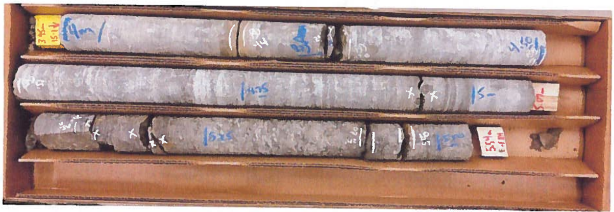
Bedrock core from BH 15-1 (dry) 3.95 m to 5.54 m depth
