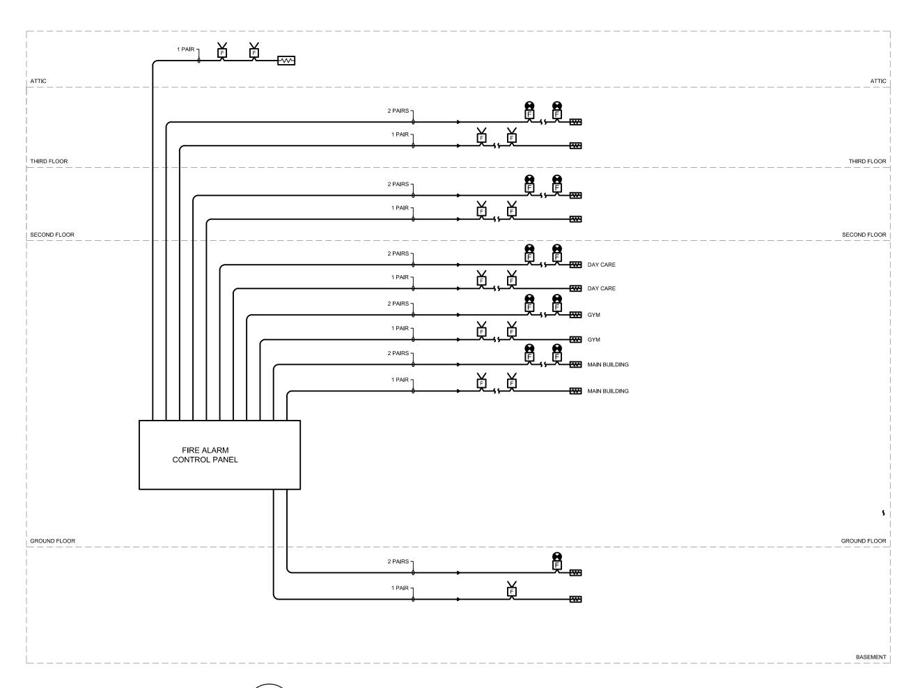
2 FIRE ALARM SINGLE LINE DIAGRAM (SIGNALISATION)
