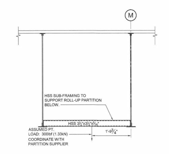
NOTE: PROVIDE HSS @ MAX 15'-0" crs. OR AS SPECIFIED BY ROLL-UP FABRIC PARTITION MANUFACTURER.
