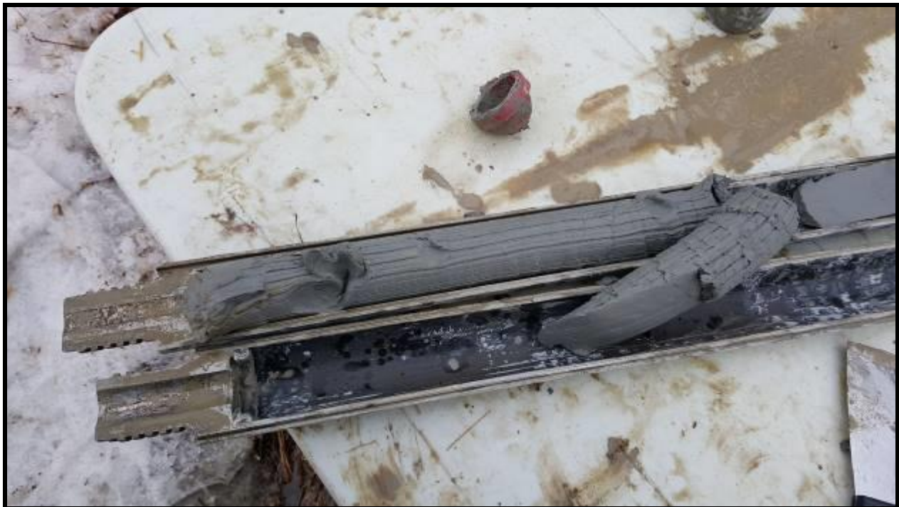
Photograph 2: View of soil sample BHMW16-2 SS7, recovered in split spoon sampling device (March 9, 2016)
