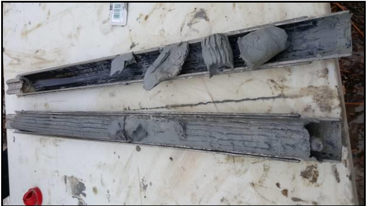
Photograph 3: View of soil sample BHMW16-6 SS8, recovered in split spoon sampling device (March 7, 2016)
