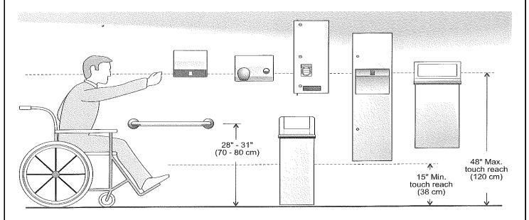
Barrier-Free access washro limided mobility and whee building codes. Mounting r the direction of reach requ mounted "above the finish a wheelchair symbol is use wheelchair symbol is also u and provide barrier-free ac Protruding objects: Object halls, corridors, passagewa Detectable objects: Pbject any amount.
