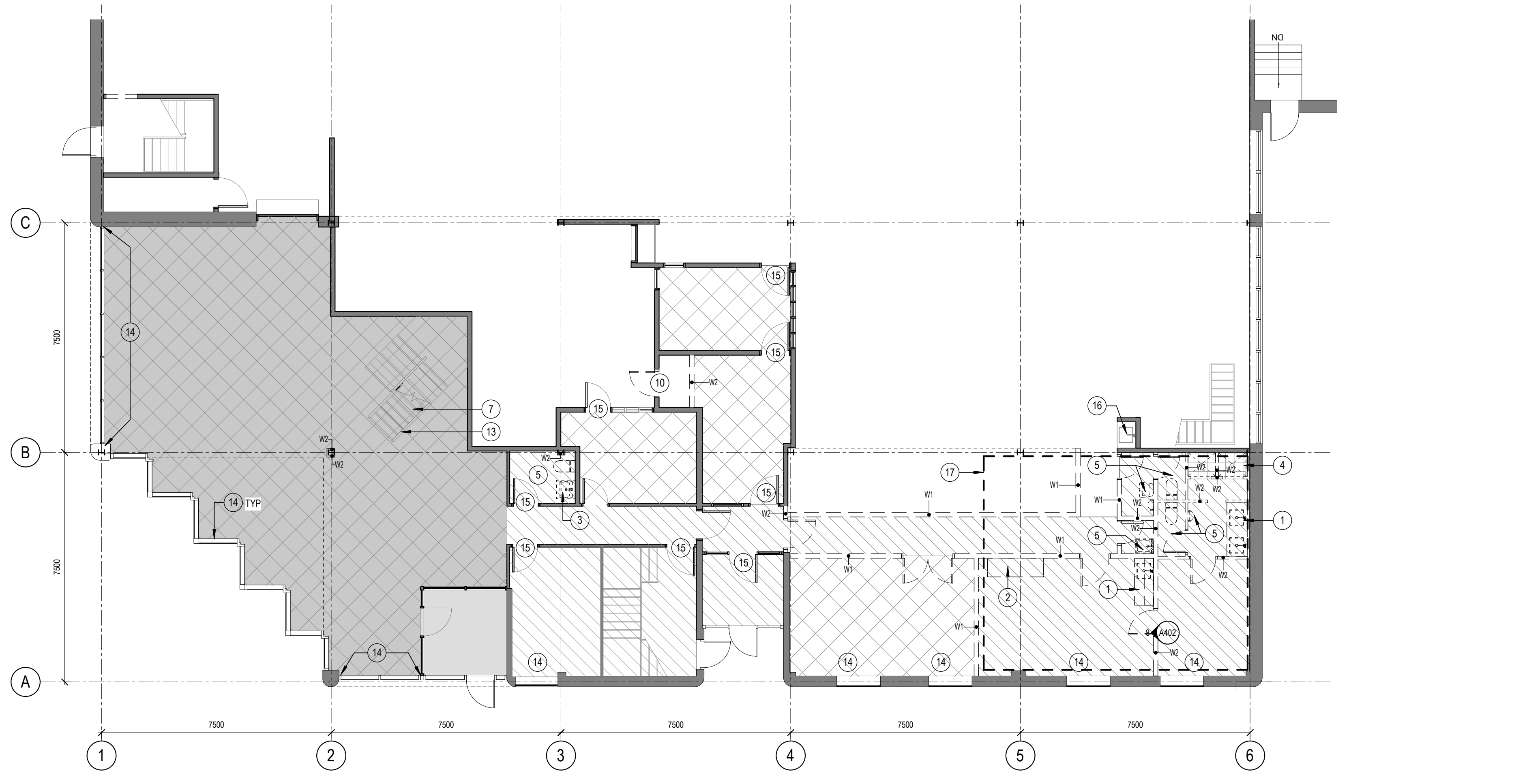
1 LEVEL 01 - DEMOLITION PARTITION PLAN D101 SCALE: 1 : 100
